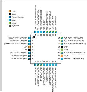
For reasons of cost efficiency nearly every pin is assigned twice. The configuration of the respective functionality takes place in software.
